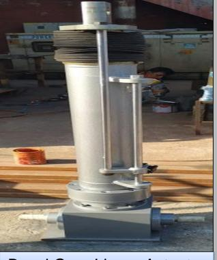
**Bevel Gear Linear Actuator**
