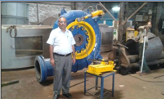
Guide Vane Servo Motors for Rukti Project
