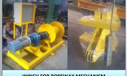
**WINCH FOR ROPEWAY MECHANISM**
