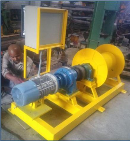
**WINCH FOR ROPEWAY MECHANISM**
